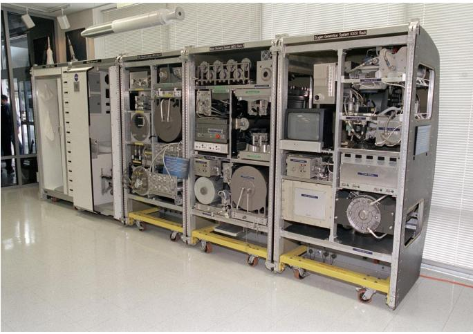
**Environmental Control and Life Support System (ECLSS)** is a system of regenerative life support hardware that provides clean air and water to the International Space Station (ISS) crew and laboratory animals through artificial means.
